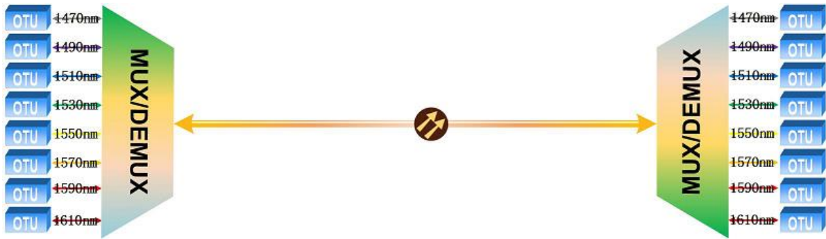
Figure 2: Multiplexing/Demultiplexing Single-fiber Bidirectional Application
