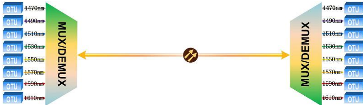
Figure 2: Multiplexing/Demultiplexing Single-fiber Bidirectional Application
